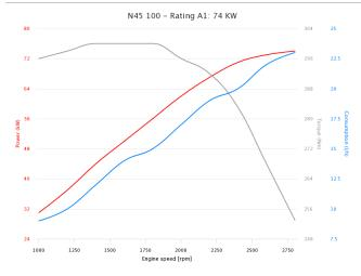
\* Net Power at flywheel according to ISO 8665, after 50 hours running, Fuel Diesel EN 590. Power tolerance 5%.
