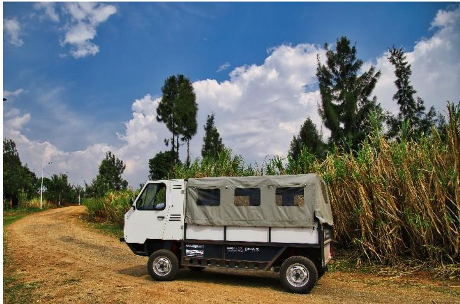
The world's first vehicle that is shipped flat packed, the electric OX truck has a cargo payload of 1,800 kg and volume of 8.8 m<sup>3</sup> and has been purpose-designed to **navigate the extreme terrain** conditions that are found in emerging markets.
