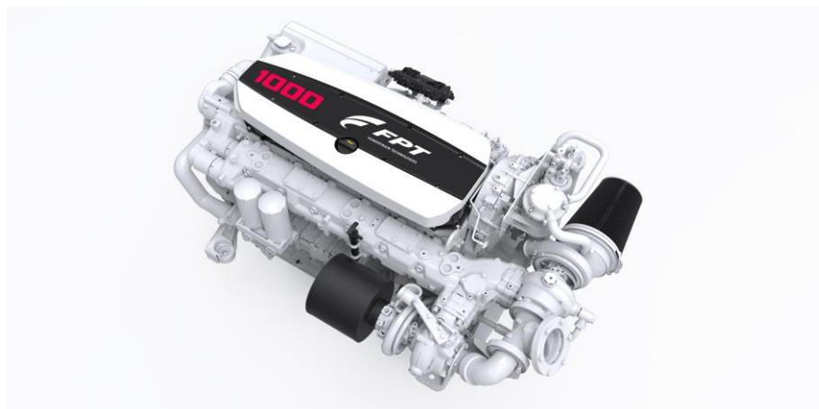
The C16 1000 was developed for light commercial and pleasure applications and distinguishes itself for providing top performance and compactness. With a 16-liter displacement and 6 cylinders in-line, its power can reach 1,000 hp at 2,300 rpm, placing itself among the best performance engines of the category. In 2018, with a specific racing configuration, this engine achieved the Guinness World Record of speed for Diesel engine boats, reaching 277.5 km/h.
