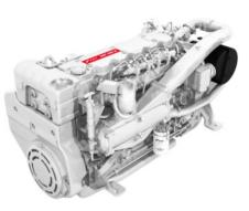
Cylinder layout: 6L Turbocharger: TCA Displacement [liters]: 6.7 Injection system: MPI Max power [hp @ rpm]: 280 @ 2800 Max Torque [Nm @ rpm]: 970 @ 1600 Certification: IMO Marpol Tier 2 Dry weight [kg]: 605 *Full specifications are available on the FPT Industrial website.*
