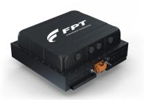
Technology: Li-NMC Nominal Energy (kWh): 37 Nominal Voltage (V): 355 Energy Density (Wh/kg): >140 C-Rate (continuous) Charge/Discharge: 1C/2C Cooling System: Water-cooled Protection: IP67 - IP6K9K Dimensions (L x W x H, mm): 925 x 854 x 310 Weight (kg): 260 Life Cycles\*: >2,500 Regulation Compliance: ECE R100.3, ECE R10.6
