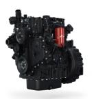
Engine Displacement (liters): 2.8 Cylinder Arrangement: in-line 4 Power (kW @ rpm): 55 @ 2500 Torque (Nm @ rpm): 375 @ 1400
