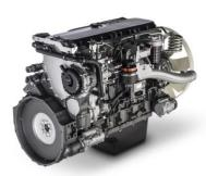
No. of cylinders / valves: 6L / 4 Turbocharger: Twin Scroll Displacement [liters]: 12.88 Bore x stroke [mm]: 135 x 150 Maximum Rated Power [HP]: 1,000 Maximum Torque [Nm]: 5,000 Dry weight [kg]: 1,150
