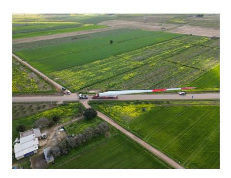
The construction of infrastructure like a wind farm involves operations with a very high level of complexity: transporting blades up to 81 meters long on a special twelve-axle trailer, with a total combined weight of over 200 tons, is certainly one of them. The maneuvers, slow and at times
