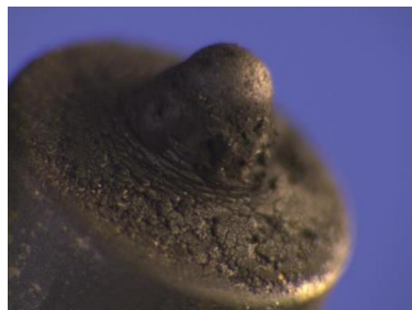
Dirty spray-orifice disk of an injector before cleaning
