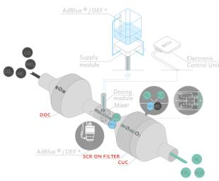
1. Diesel **Oxidation Catalyst** NO → NO. HC, CO and PM oxidation
