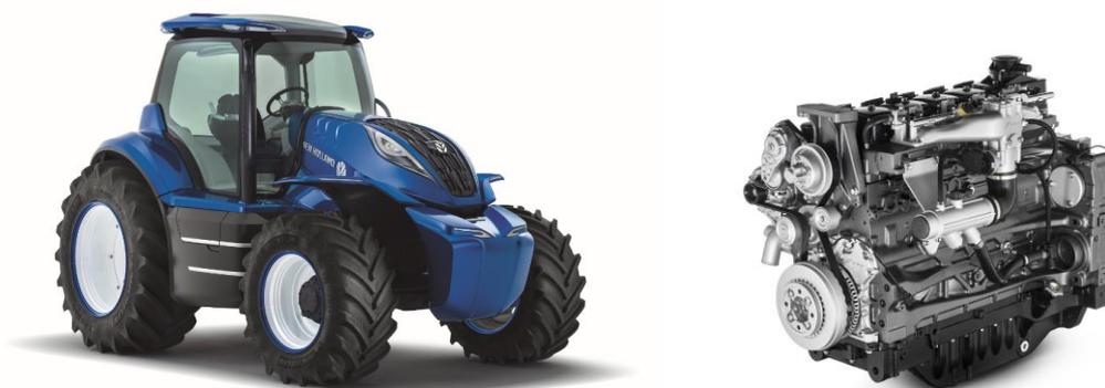
*New Holland Agriculture methane powered new concept tractor and FPT Industrial 6 cylinders NG engine*
